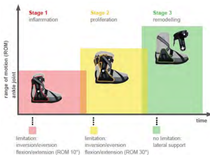
Figure 1. The Ortho Tri-Phase™ ©Künzli semi-rigid brace. The diagram depicts the phase adapted concept of the Ortho Tri-Phase according to the healing stage. Range of motion (RoM) is initially limited to 10° of flexion/extension and can be gradually increased, as shown above, without the need to change the device. (Graphic with Permission of Künzli/Switzerland).
