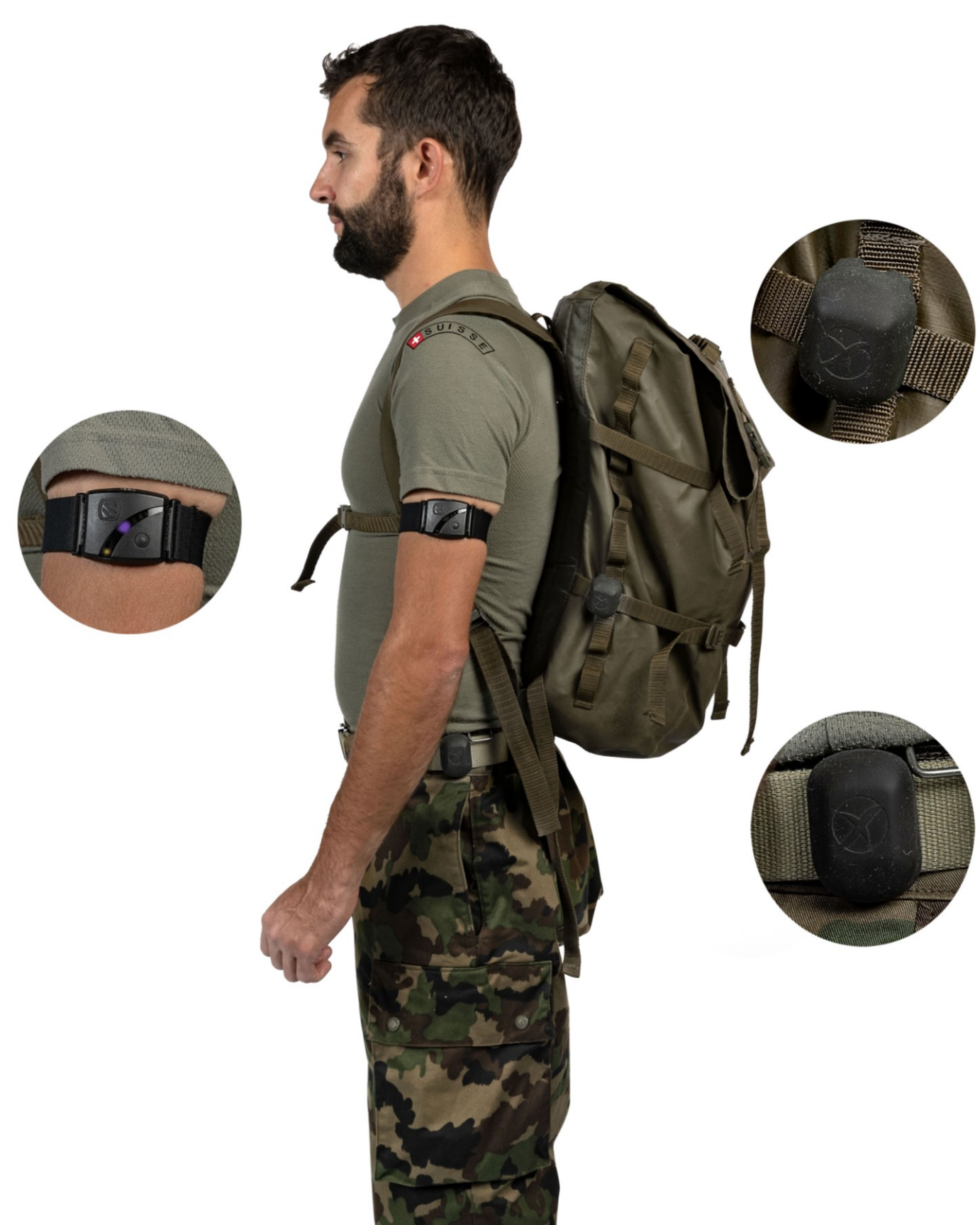
Figure 1: Soldier wearing a heart rate monitor (Rhythm24; Scosche Industries Inc., Oxnard CA, USA) on the upper arm, an accelerometer (Axiomo PADIS 2.0, Axiomo GmbH Biel, Switzerland) each on the hip and the backpack.
