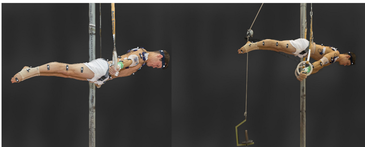
Figure 3. Test conditions for static exercises. The swallow (left) and support scale (right) exercises were performed with maximum resistance for five seconds. These examples show the use of additional weight (left) and the pulley and counterweight (right).
