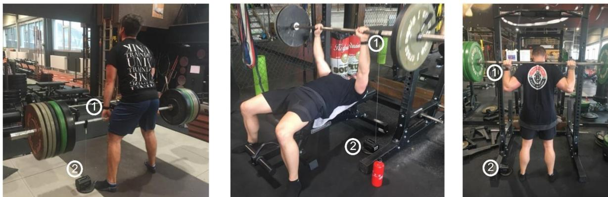
**Figure 1.** Measurement devices used during testing: (1) Apple Watch Sport, (2) GymAware PowerTool.
